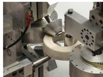
**Fig. 3** Flexible Ring Rolling Machine
