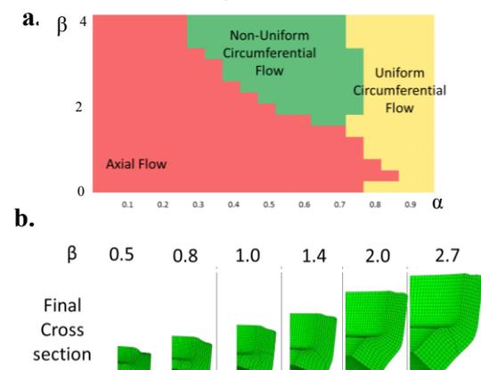
**Fig. 7** Prediction of flow patterns: a. Upper Bound Map, b. FEM simulation
