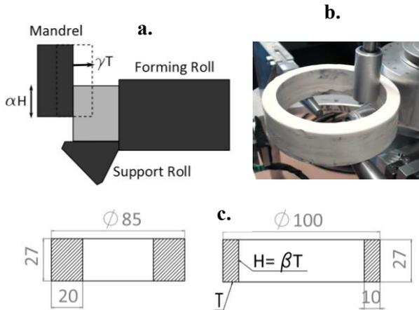
**Fig. 4** a. Toolpath Parameters (inner profiling) b. Experimental Set-Up c. Preform Geometry
