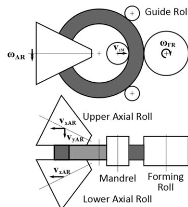
**Fig. 1** Radial-Axial Ring Rolling Machine
