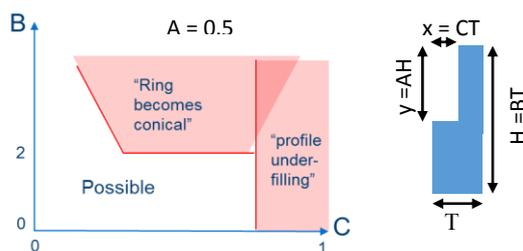
**Fig. 8** Operating Window for L-Shapes
