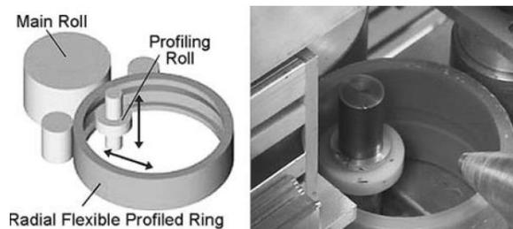
**Fig. 2** Flexible Radial Profile Machine [6]
