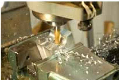
Machining aluminium and making swarf
