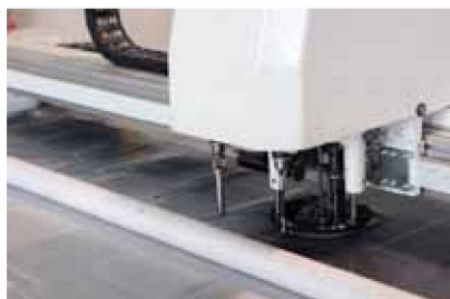
CNC machine cutting and perforating fabric
