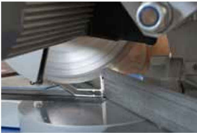
Cutting aluminium with a circular saw
