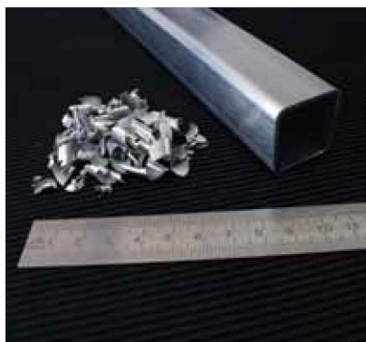
Early solid bonding trials to create a box section
