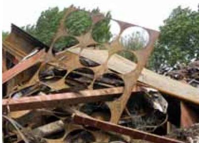
A typical 'skeleton', left over after blanking
