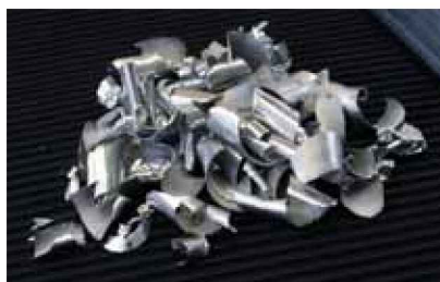
Aluminium machining swarf
