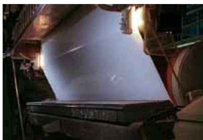
Wet end of a paper making machine
