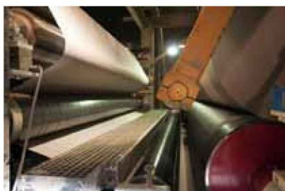
Dry end of a paper making machine
